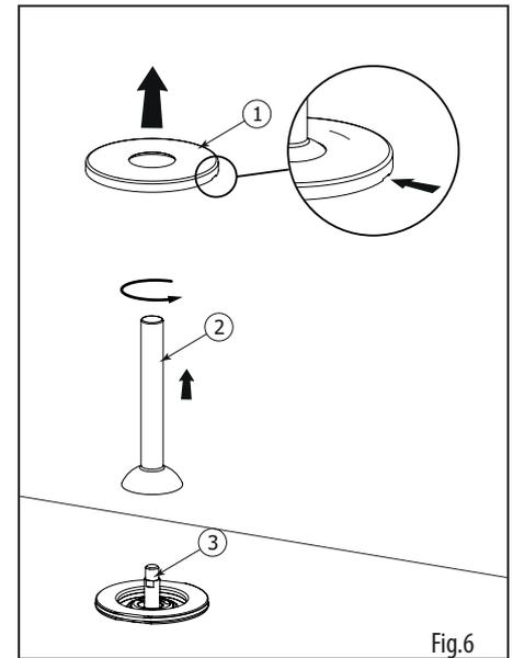
Start by shutting off water supply lines and then turning on the water to drain the faucet. To replace the cartridge (3), remove the decorative ring (1) using a small flat screw driver and pull. Then unscrew the lever handle (2) to have access to the cartridge (3).
